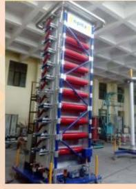
1000kV, 100kJ Impulse Voltage Generator
