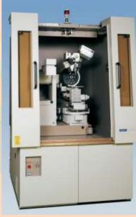
Residual stress test - XRD based
