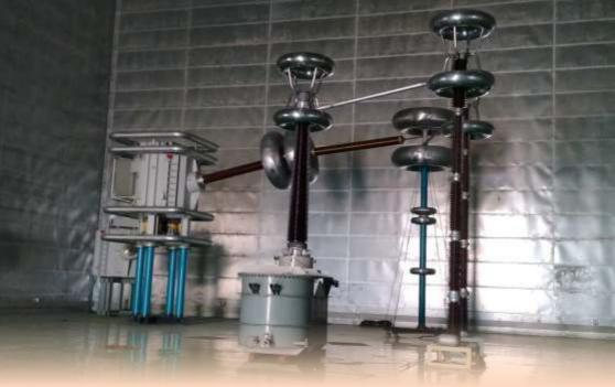
420 kV OIP Condenser Bushing undergoing Partial discharge and Long duration AC voltage test
