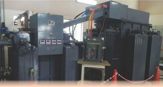
30 V, 10000 A Current Source for Accuracy Test on CT
