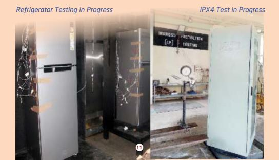
**Ingress Protection Testing Laboratory:** The lab is equipped with dust test chamber to perform IP 5X and 6X to accommodate the test panels/ samples of size up to 2.2 m x 1.8 m x 2.5 m (W x L x H) and water test facility to perform tests ranging from IP X1 to X8 test. The Lab undertakes the tests ranging from IP 11 to IP 68.
