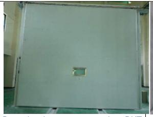
Dust chamber to accommodate DUT of size upto 4.5\*4\*4m (WDH)
