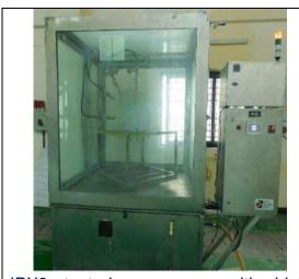
IPX9 test in progress, with high temperature and pressure.
