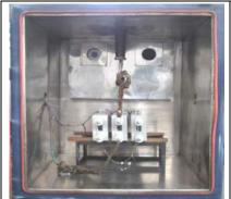
Arrangement for Thermal Stability Test on 1032kvar 12.025kV, Int.Fuse capacitor unit
