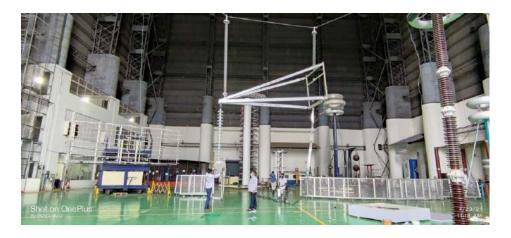
Lightning Impulse voltage withstand Test, Dry & wet Switching Impulse Voltage withstand Test, Dry & Wet and Power Frequency Voltage withstand Tests on 132kV /23L VMCC FRP Composite Cross Arm
