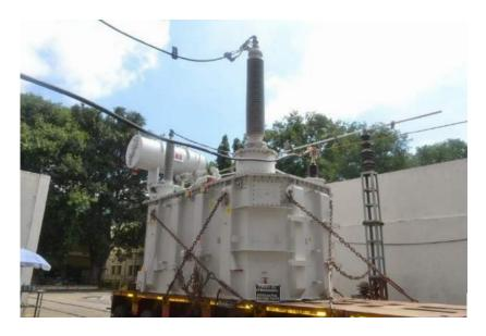
Dynamic ability to withstand short circuit test on 53.33 MVA,  $220/\sqrt{3}/132/\sqrt{3}/33$  kV single-phase Transformer
