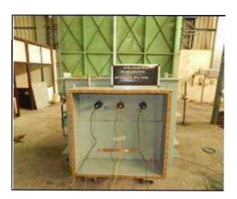
Temperature-rise and Determination of sound level tests on 1500kVA 22000/433V Three Phase Oil Immersed Distribution Transformer
