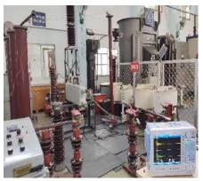
Arrangement for Short Circuit Discharge test 949.81kvar, 6.944kV, Internal Fuse Capacitor unit
