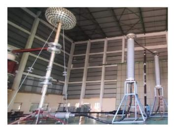
Type Test on 1C X 2500 Sqmm, 400 kV Cable System as per IEC: 62067
