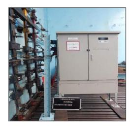
Short circuit withstand test on 500V 400A 6 Way LV Feeder Pillar
