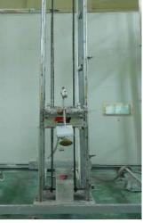
IP X3, X4, X5 and X6 test device with an auto movement of test nozzles
