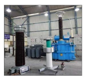
Accuracy test on 220kV (ratio: 220kV/ $\sqrt{3}$ :110/ $\sqrt{3}$ , 10VA, 0.2 class) Inductive Voltage Transformer
