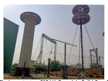
Critical Impulse Flashover test on 525 kV, Porcelain Solid Care Post Insulator
