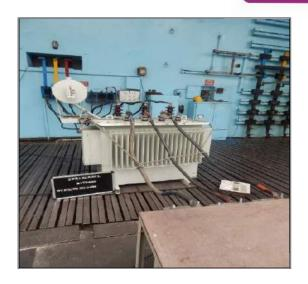
Ability to withstand the dynamic effects of short circuit, Thermal ability to withstand short circuit & Temperature Rise tests on 200kVA 11000/415V & 250kVA 11000/415V Three Phase Distribution Transformers
