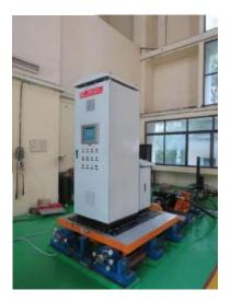
Vibration testing of Local control panel and Remote Control Panel of Coal Feeder
