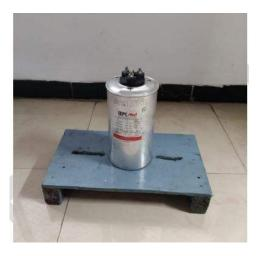
A view of the tested 50kvar, 525V, 3 Ø, 50 Hz, MPP type LV Capacitor after completion of Destruction test
