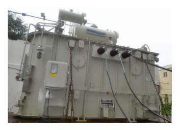
Dynamic ability to withstand short circuit test on 16/20MVA, 33/11.3 kV three-phase Transformer
