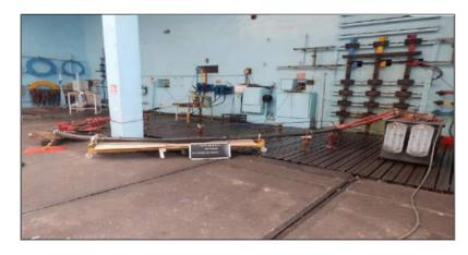
Thermal short circuit test at 20kA rms for 1 second through screen & armour on 3 x 240 sq.mm Copper conductor, XLPE insulated PVC sheathed 18/30kV Cable with accessories (Heat Shrink Indoor Termination, Outdoor Termination and a straight through joint)
