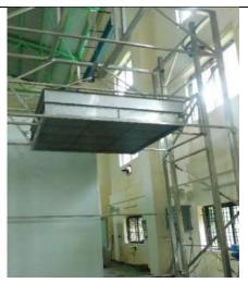
IP X1 and X2 test device
