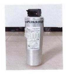
A view of the tested 30kvar, 440V, 3Ø, MPP Type LV Shunt Capacitor
