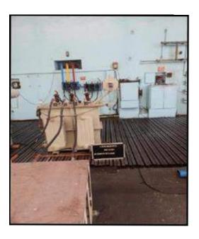
Ability to withstand the dynamic effects of Short Circuit & Temperature Rise tests on 200kVA 11000/415V & 250kVA 11000/415V Three Phase Distribution Transformers
