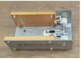
A view of the discharge resistor
