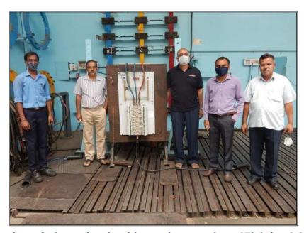
Verification of short circuit withstand strength at 17kA for 0.25 s with 34 kA peak on main bus bars, at 10.2kA for 0.25 s with 20.4 kA peak on neutral and earth bus bars on 415V 160A 12 Way LV Distribution Board
