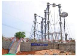
A View of ± 1200 kV DC Test System
