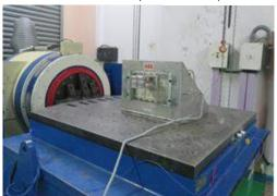
Vibration, Shock, Bump and Seismic tests on Electromechanical Auxiliary Relay
