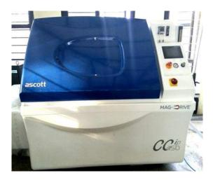
**Cyclic Corrosion Test Equipment**
