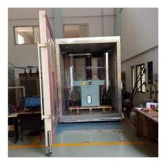
A view of the tested 36 kV, 2000A, 31.5 kA, Outdoor VCB
