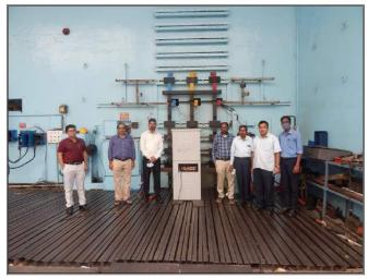
Verification of short circuit withstand strength test at 31.5kA for 3s with 66.15 kA peak on main bus bars & 18.9 kA for 3s with 37.8 kA peak on neutral bus bar on 400V 1600A Ground mounted LV Metering KIOSK
