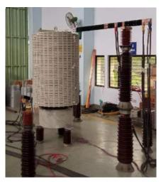
A view of the line-trap test in the Laboratory
