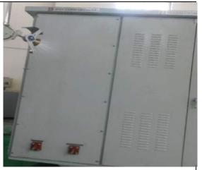
IP X4 test in progress with an auto movement of test nozzles
