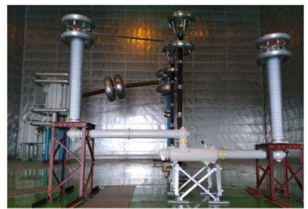
Power Frequency Voltage Withstand test on 400 kV, 4000 A, 63 kA GIS
