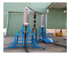
Cable outdoor terminations connected for heating cycle voltage test
