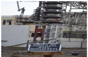
Power Arc test on 25kV composite insulator
