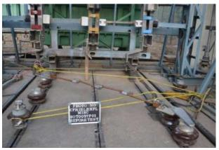
Short time current test on Burndy fired wedge connectors for panther conductors
