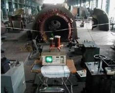
Partial Discharge test on 110 MW Turbo Generator
