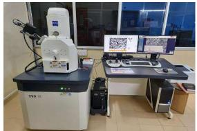
Advanced Scanning Electron Microscope with EDX facility
