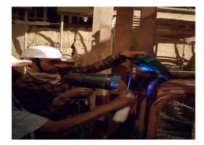
Root Cause analysis of IP Turbine Control Valve of Unit No.2 (660MW) carried out at Prayagraj Power Generation Co. Ltd., Allahabad, U.P. The IP Control Valve of RHS, Unit No.2 (660MW) suddenly failed during running condition. All flange bolts got sheared off and the turbine which was running at 490 MW got tripped on high vibration.
