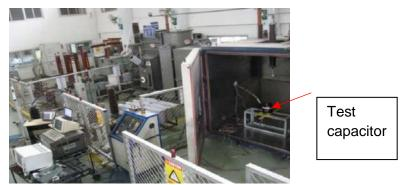
Test set used for energizing test capacitor with HVDC superimposed with HVAC current
