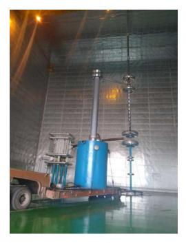
800kV RIP Transformer Bushing undergoing Partial Discharge test
