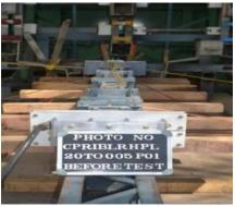
Short time current test on 1000V, 1600A Sandwich busway
