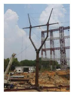
Testing of 400 kV S/C "Y" shaped steel monopole
