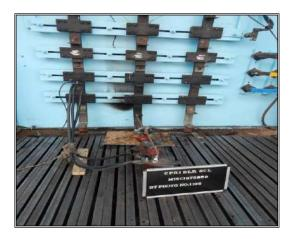
Short-time current test on Ground Clamps
