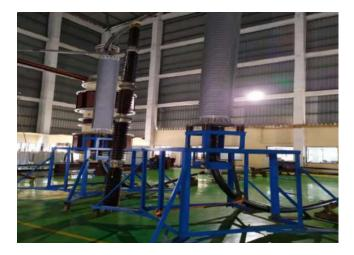
Extension Pre-Qualification test on 127/220 kV XLPE Cable with accessories
