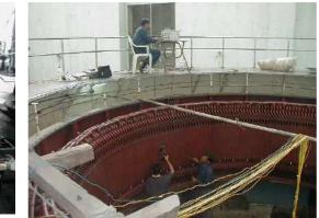
ELCID Test on Hydro Generator
