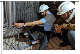
Figure.2: Detection of Magnetite at tube bends
